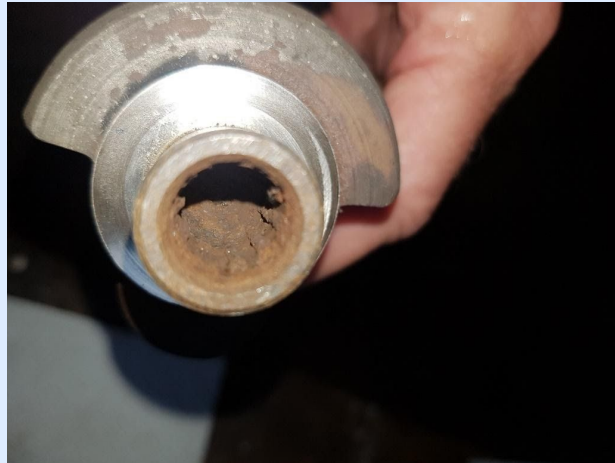
The socket on the end of the crankshaft showing why the driveshaft was jammed.
