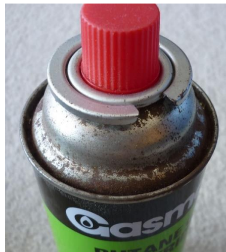
It Doesn't Take Long for these Cannisters to get Rusty, Especially in a Marine Environment
