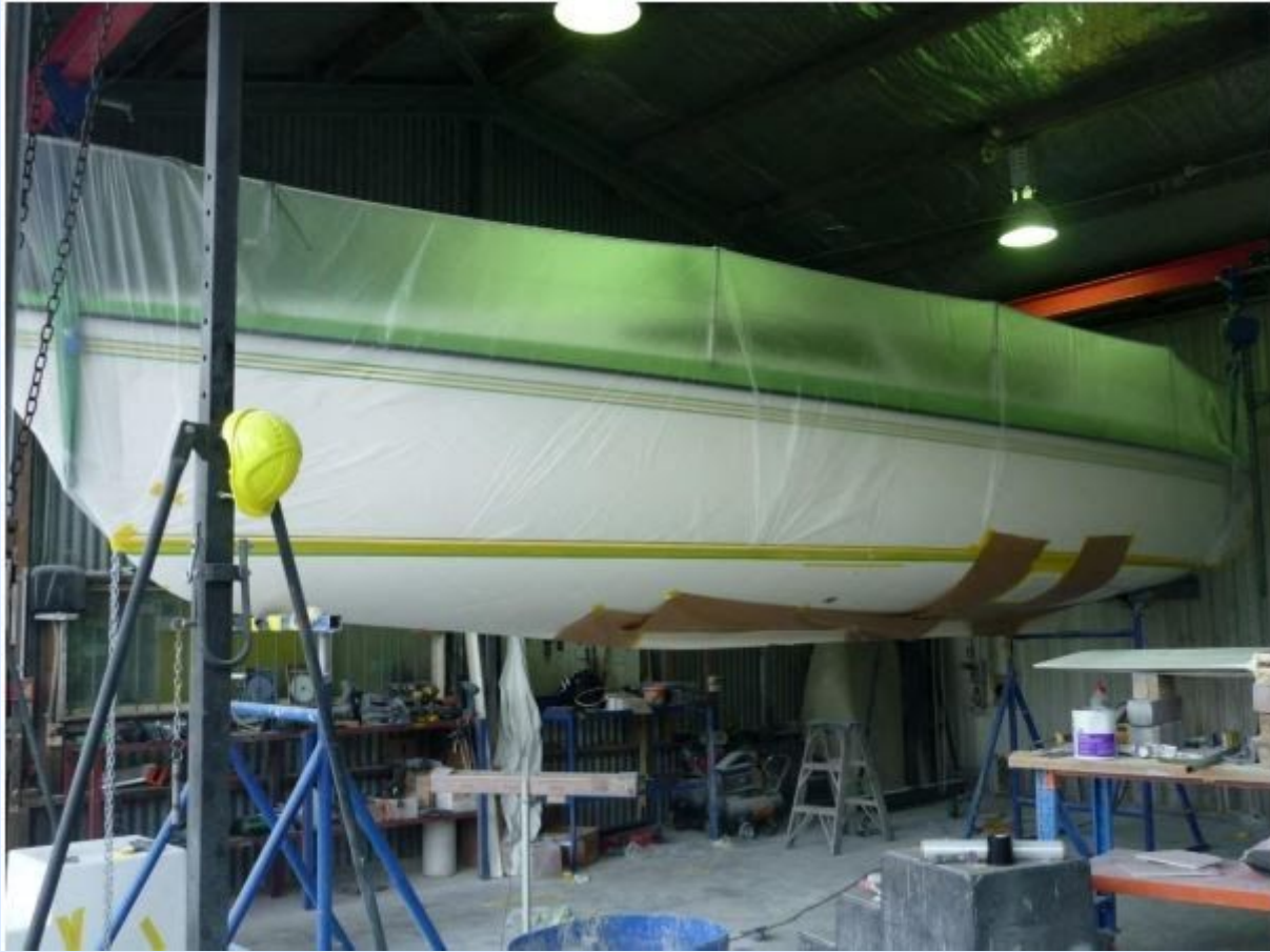
All ready for some spray touchups
