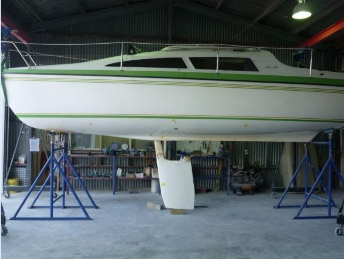
Charley up in the air with the keel lowered and about to be removed
