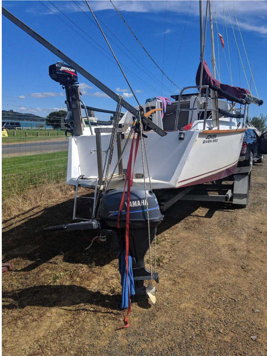
The Compound gantry crane system. It's basic but it works, is quick and easy to use, and is usually way better than trying to manhandle a heavy motor on or off your boat
