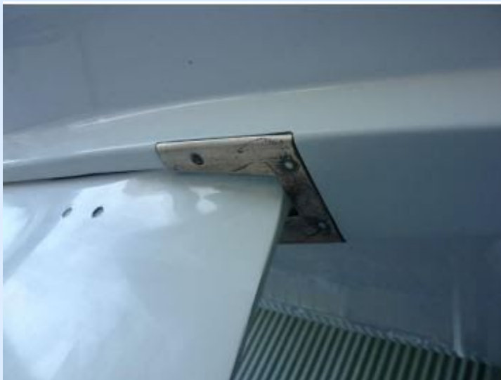
Aft end of the keel showing the keeper plate – all rejuvenated and back together
